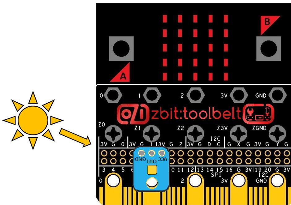
*This zbit:toolbelt example shows you how to plug the Adafruit Log-Scale Analog Light Sensor onto zbit:toolbelt and use it to display the ambient light level as a bar graph on your micro:bit*
